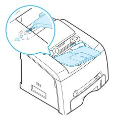
Fold out the extender, if necessary.
